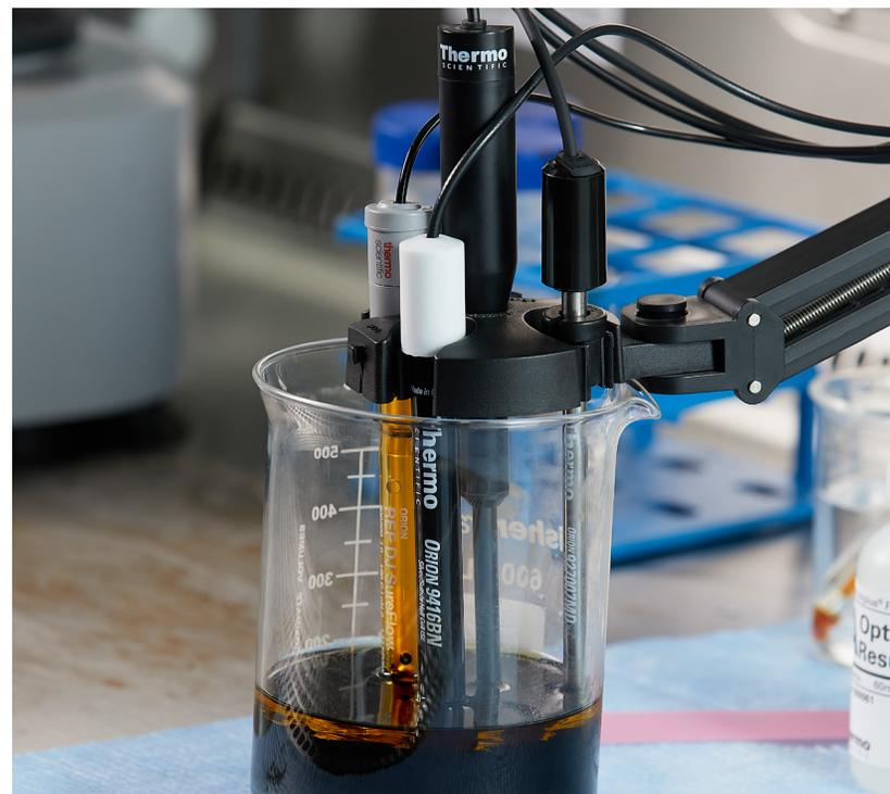
**Low level measurement** is a similar method to direct measurement. It is recommended when the sample is not in the linear response range. A minimum 3 point calibration is recommended to compensate for the non-linear response. Calibration is performed in one beaker reducing the chance of cross contamination of the standards.
