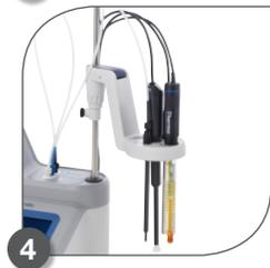
Pair with premium ROSS pH, Orion redox or ion selective electrode technology to provide a complete measurement system optimized for accurate, reproducible sample analysis.
