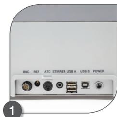
Titrator connections have clearly labeled functions, including three USB ports for printer, USB flash drive, and computer software connections.
